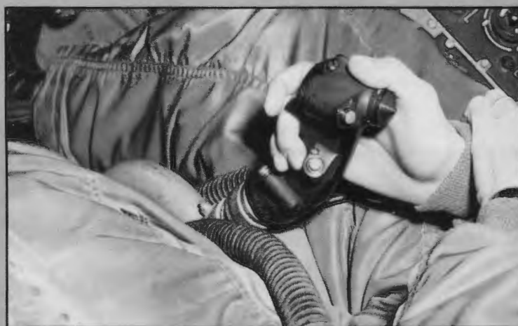
Aft stick movement possible with clip removed and hoses rerouted.
