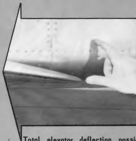
Total elevator deflection possible with clip installed.
