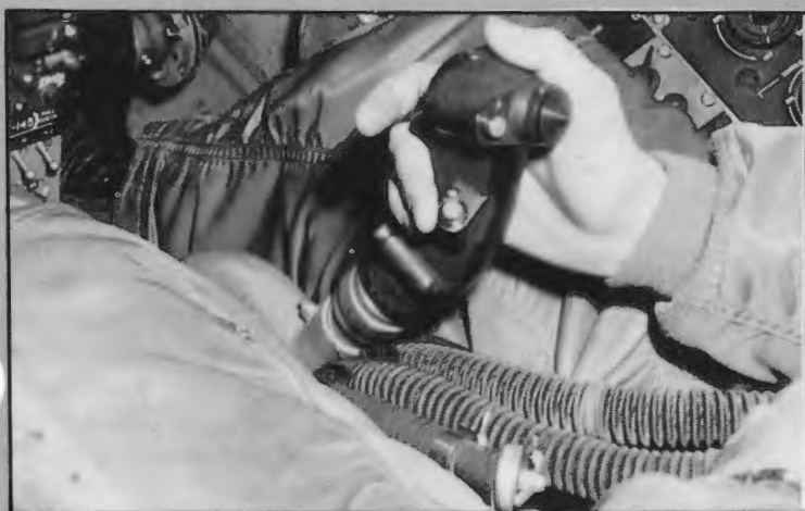
Aft movement of stick restricted by hoses with seat full up.
